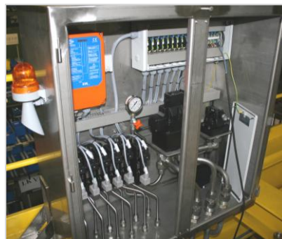
Control box with receiver as electro-hydraulic interface
