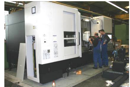
Right now technical engineers of the manufacturer are installing the multi-function-lathe.
